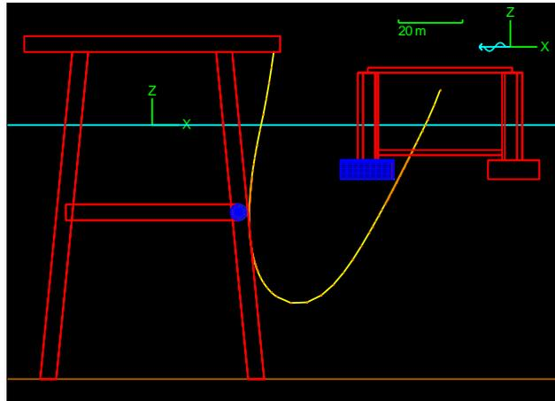
A cable catenary is suspended between a semi-submersible rig and fixed jacket. It is analysed in a random sea.
