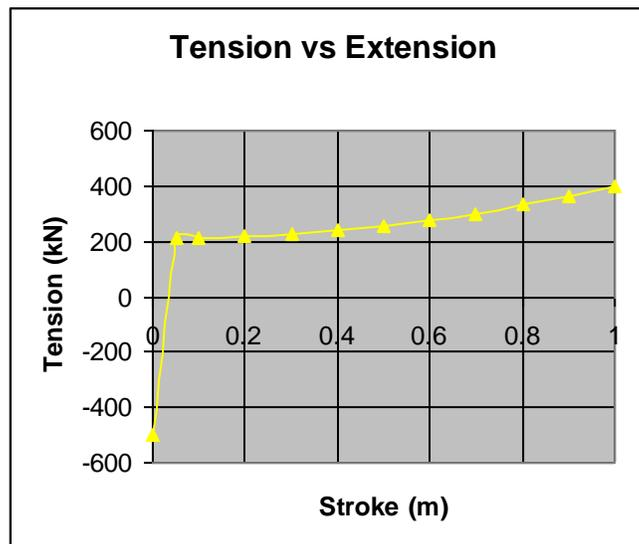
The other part of the control mechanism is the damping of the motion. The CRANEMASTER mechanism provides more damping on the return than on the extension. This has been reproduced by applying non-linear damping to the *Passive Heave Non Linear* link.
