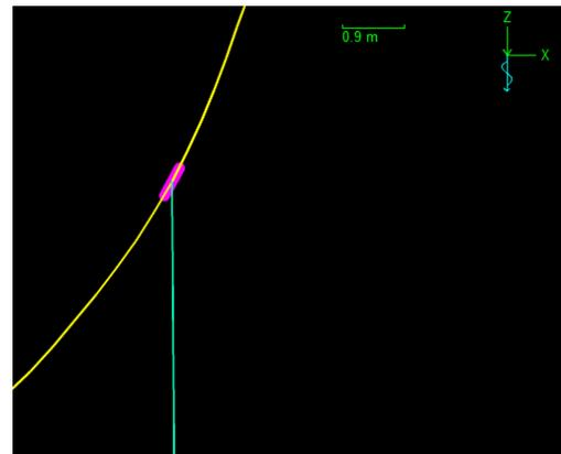
Open the *attachment types* data form via the *attachment types* button at the bottom left of the line data form to see the clamp settings. The physical properties are for those of the steelwork alone. As for the buoyancy modules discussed in the lazy wave example, the clump attachment should only contain loads that are additional to the riser's loads.
