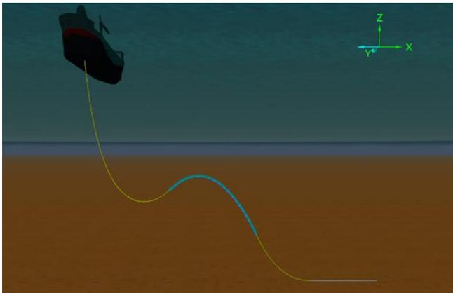
Both risers have the same end connection settings and the same number of sections. As with the simple catenary model, refined segmentation has been applied where needed.
