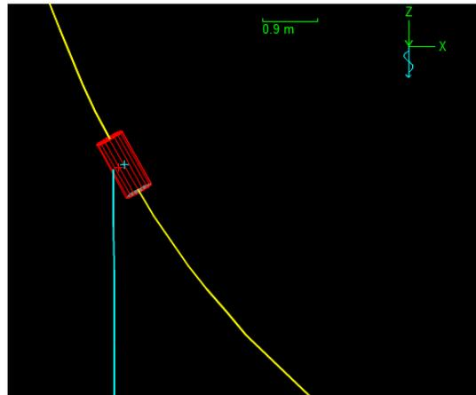
As the clamp is 1m long, each riser length has been shortened by 0.5m so the total length is still 232.5m. Hydrodynamic properties assigned to the buoy exclude any contribution from the clamp itself but include contributions from the riser to allow comparison with the simpler clamp method above.
