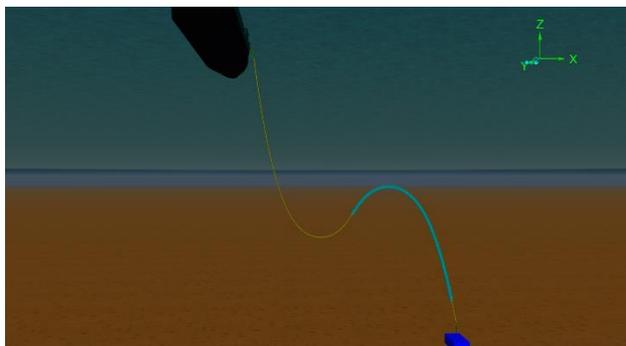
In each group, the riser is built in a similar manner as for a lazy wave (discussed previously), however the 'steep' configuration means that the lower end is vertical rather than horizontal when it reaches the seabed.
