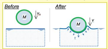
A cylinder (mass M) approaching flat water with a velocity,  $v_0$ , (see above) has a momentum of  $M.v_0$ . On penetrating the water, the momentum is then  $(M + m_a)v$ , where  $m_a$  and v are the mass and velocity of the moving fluid particles<sup>1</sup>. Conservation of momentum gives  $M \cdot v_0 = (M + m_a)v$  and the force exerted is equal to the rate of change of momentum (Newton's second law):
