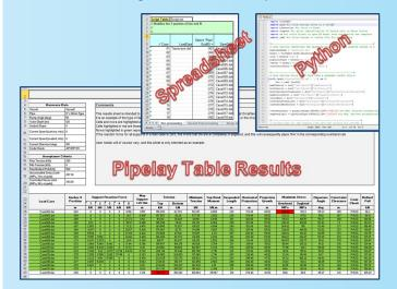
done programmatically using some *python code* (these files are now distributed as standard examples). With the Spreadsheet approach you have to consider a range of laybacks to encompass both the min and max possible laybacks. The python approach is more robust and automatically looks for the min and max laybacks for you, and then automatically steps between these!
