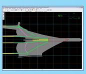
Superwide Failure OrcaFlex models the consequence of rigging failure on what is otherwise a simple 2 streamer symmetrical model.
