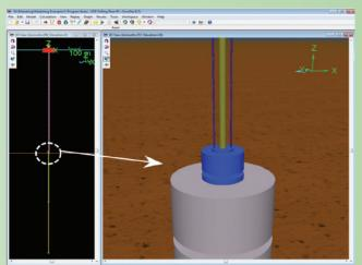
Here the Choke and Kill lines on a drilling riser are explicitly modelled clamped to the marine riser. The drill string is not visible but runs inside the marine riser through the Flex Joint, BOP and sub-seabed casing.
