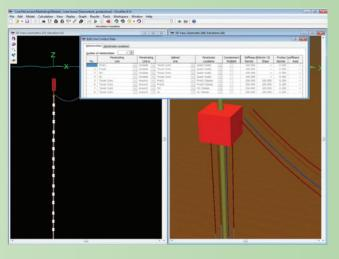
The riser tower has a central core with 4 production lines around it. Relationships 5-8 set the core's penetrators around the production lines to represent clamps. Strictly the Relationships I -4 are not needed as we don't expect the 4 production lines to contact the tower core... but just in case ;-).
