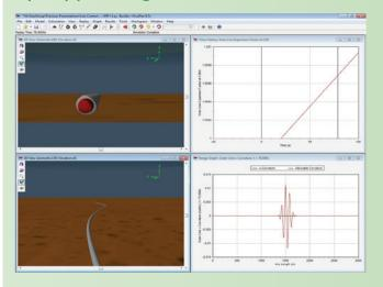
This model shows a classic pipe-in-pipe system. OrcaFlex is explicitly modelling one line inside another. The inner line is set with an expansion factor representing thermal expansion. The resulting buckle in the line is clearly shown.
