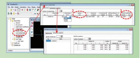
f) A **'contained'** line will be shielded from the external fluid forces (and from contact with elastic shapes and the seabed). But the shielded section of a contained line sees fluid effects from the contents fluid and contents motion in the containing outer line.
