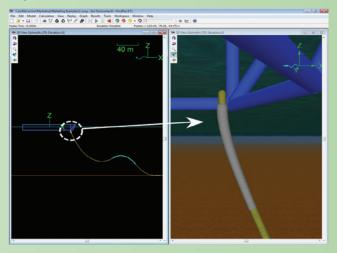
Here the bend stiffener is modelled explicitly as a separate OrcaFlex Line with a tapered profile. The Line Contact Relationships call for the riser to be inside the stiffener, and this is achieved in statics. Friction between the riser and the bend stiffener is optional. The dynamic run then proceeds as normal. Results can be obtained for both lines separately.
