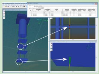
This model shows an SCR on a SPAR with 3 guide tubes and a stiffener on the keel, all using the Line Contact model. The Relationships are shown inset. These are quick and easy to setup and now make statics convergence very much easier than before.
