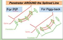
specified. So one line can interact with lots of others, eg., an SCR through guides; One line slipping off another and then interacting with a third line; a line inside a line inside a line....., etc.
