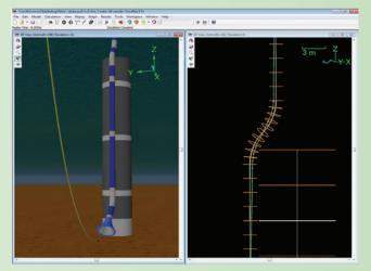
J-tube modelled as an OrcaFlex line with pre-bend so it responds to the loads acting on it from the pulled-through riser. The J-tube is clamped to the structure also using the Line Contact model. Friction and large scale relative motion now mean that the Line Contact model is the preferred way to model J-tube pull-ins.
