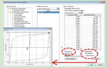
There are several options for setting the bend stiffness of a Line. The simplest is a constant value giving a linear elastic response. Alternatively, a non-linear elastic response can be specified, as shown in the curve OA in the above screenshot. For composite cross-sections (flexible risers, umbilicals, etc), selecting the Hysteretic checkbox (highlight I) means the full non-linear hysteretic curve, as shown, will be used.
