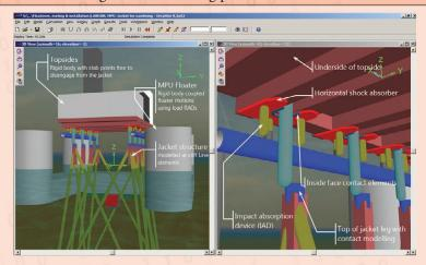
The tops of the jacket legs also include contact elements, allowing potential intermittent re-contact between the lifted jacket leg and the remaining jacket structure to be modelled.
