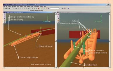
The rollers and lateral restraints are single segment OrcaFlex Lines used as contact elements. Clearances are continuously monitored – zero leading to a contact and the resulting reaction feeds into the post contact behaviour. The contact modelling on OrcaFlex, long recognised for its robustness and versatility, easily handles this.
