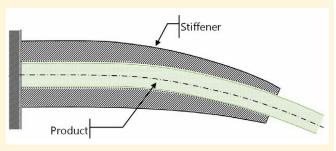
(arclength z=0m in the example above). The product line is then set up as normal on the line data form - by doing this the product line runs through the stiffener. Taking this approach means that we can get results separately for the Stiffener and the product – particularly good for doing the fatigue analysis of the product alone and it also means the product can have non-linear elastic or hysteretic properties.
