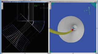
Other applications include pull-in to manifolds and wellheads, pull around turning points or anything else that might generate a capstan load. Another key application is to model the frictional forces between a line and a mid-water arch. A novel application is the ability to create a seabed with a number of shapes. Each shape can then have different friction coefficients representing different areas of seabed soil with different friction coefficients.
