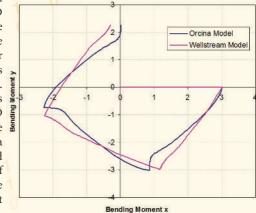
The models show different predicted trajectories for the bend moments. But these, and the final bending moment values predicted, are quite similar. This gives confidence in the way 3D bending is handled, as only the momentcurvature data is common to both models.
