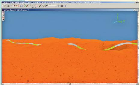
Data entry is simply a series of x, y and Z coordinates, and OrcaFlex lets the user select between Linear or Cubic Polynomial interpolation. For most situations we recommend the Cubic fitting which results in smooth interpolation. The linear method is best suited to the case where you only have depth and slope information at anchor points – you can then effectively create a series of flat sloping seabeds, one for each line.
