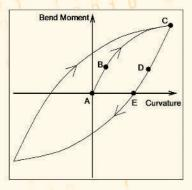
axially within the structure. This slippage reduces wire tension (compression) increase at the outside (inside) of the bend, thereby reducing any further increases in the bending moment. This effect decreases the slope of the moment-curvature curve. (BC)
