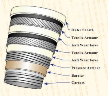
What is Hysteresis: Unbonded flexibles have concentric layers, with some helically wound tensile armour wires. On bending, each layer contributes to the total bending moment. The non-tensile layers generally bend with the pipe with a non-hysteretic behaviour. However, bending of the tensile wires produces tension which in turn tries to slip the wires within the structure. This is resisted by friction and leads to hysteretic behaviour.
