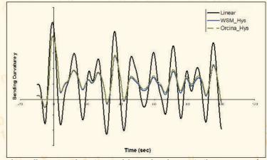
The Wellstream and Orcina models produced very similar responses for curvature in the TDZ (see graph above). Compared to the linear stiffness model, a considerable reduction in the curvature amplitude is predicted by the two hysteresis models, significantly impacting fatigue results.
