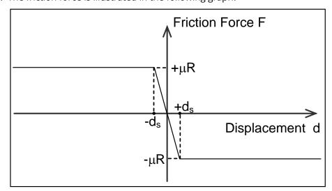
The distance  $d_s$  over which the friction force is ramped from zero to  $\mu R$  is therefore given by  $d_s = \mu R/(K_s.A)$ . It is small if a high seabed shear stiffness is specified, but larger if a low stiffness is specified. If the object was lying on the seabed with no other forces applied then its 'free'
